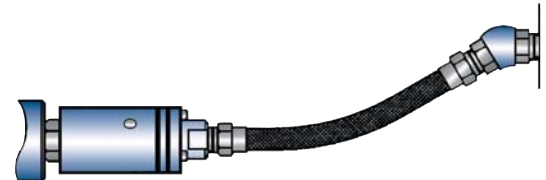
Hose should be a minimum of 300 mm long.
